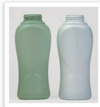
Left: Prototype made of a 50/50 blend of virgin and recycled resin Right: Bottle using recycled material with white-color coating of virgin plastic
