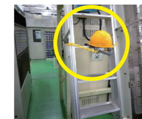
Example of a good initiative at Nippon Closures' Okayama Plant: by equipping ladders with helmets and chains, the plant is able to reduce the risk of falls and restrict unnecessary access to high-up work sites.
