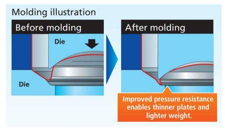
[Reference] Illustration of a can bottom being formed using CBR
