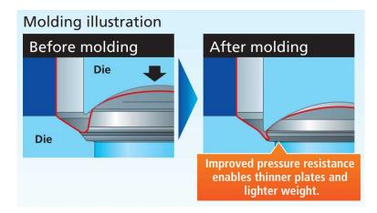
Compared to conventional can-making technologies, CBR is an innovative technology that offers both quality and weight savings, such as higher can bottom pressure resistance strength, and also leads to a reduction in greenhouse gas emissions due to the reduced use of aluminum materials.
